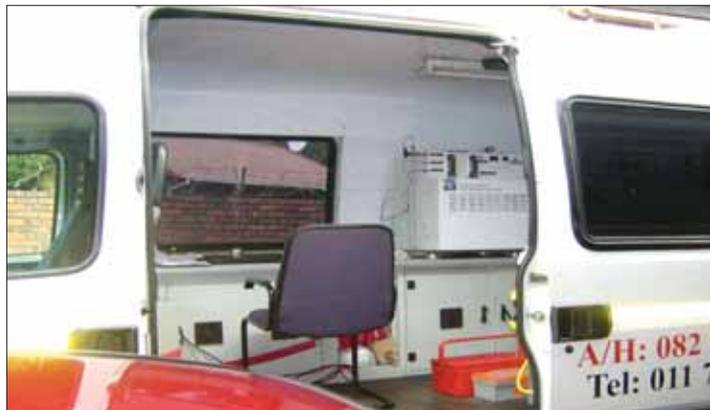
Fig. 4 a, b, c: Test van containing PFT detection equipment.
